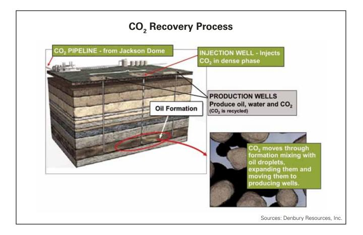
those developments were found in Colorado, New Mexico, and Arizona. Developing the  $CO_2$  resources required drilling wells into geologic formations that contain  $CO_2$ , which was then transported via pipeline to the oil fields in West Texas. The increase in oil prices in the 1970s supported the development of this infrastructure.
